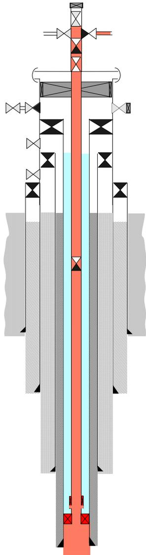
Figure 2 – well schematic, cemented to surface
