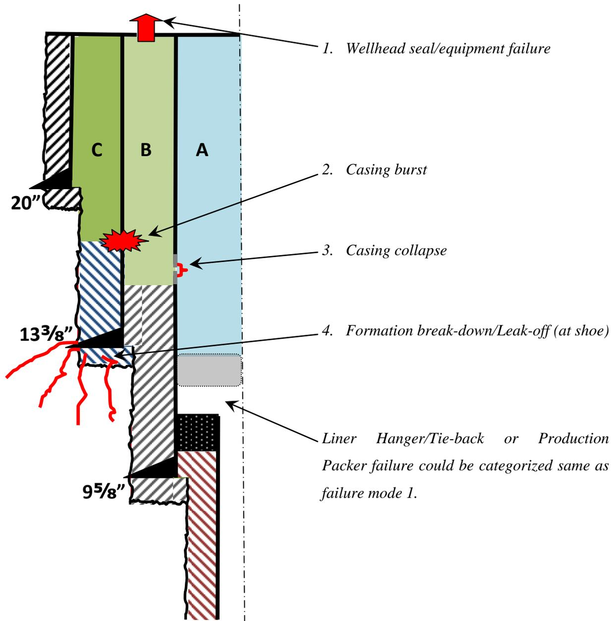
Figure 5 – typical annuli failure modes
