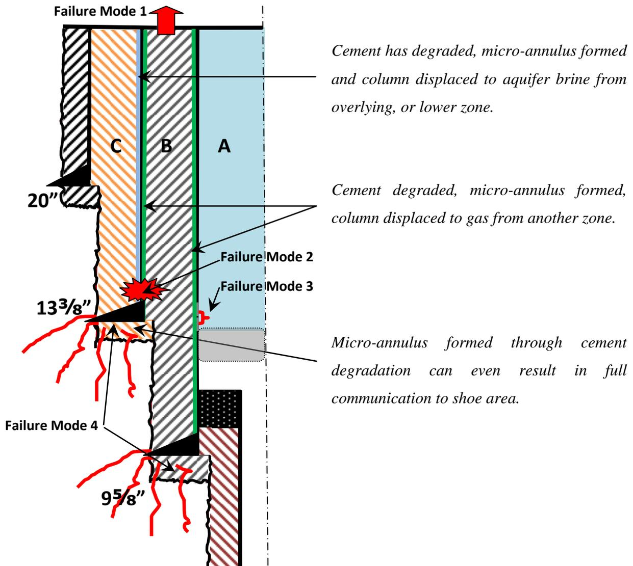
Figure 6 – fully cemented ageing well, annuli failure modes
