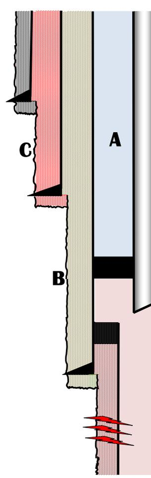
Figure 3 – well schematic, fully cemented casing
